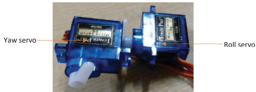
Fig.1 The yaw-roll servo arrangement in the newly designed spoon actuator
